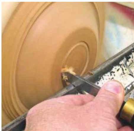
▲ Pic.8 Once you have marked up the size required, forming the chuck holding spigot is a simple matter of just cutting in about 6mm with the parting tool. Using a foot instead of a recess will help with the shape of the bowl
